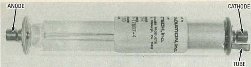
FIG. 6—A HELIUM-NEON laser tube. The cathode end can be identified by the small tube used to fill the laser tube with gas.
